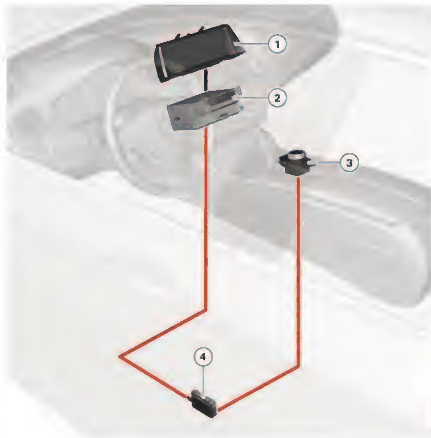
Signal path, controller with touchpad
